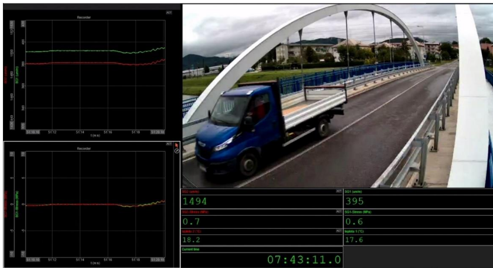
Vehicle crossing the bridge: on the left side there is data from sensors on graphs (green sensor is the belt voltage on the right, red on the left), below the image of the vehicle are their numerical values and data from temperature sensors
